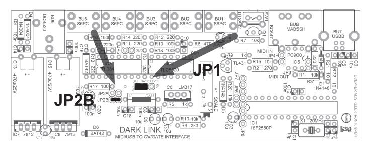
To generate a switch trigger, the jumper (JP1) has to be taken off.
