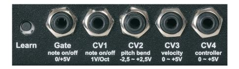
Depending on the incoming MIDI data (note on/off, notenumber, pitch bend, MIDI controller, velocity), the interface will generate:
