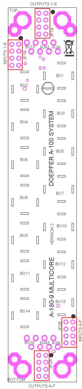
From version 2 four additional pin headers are available to enable internal default connections of two modules:
