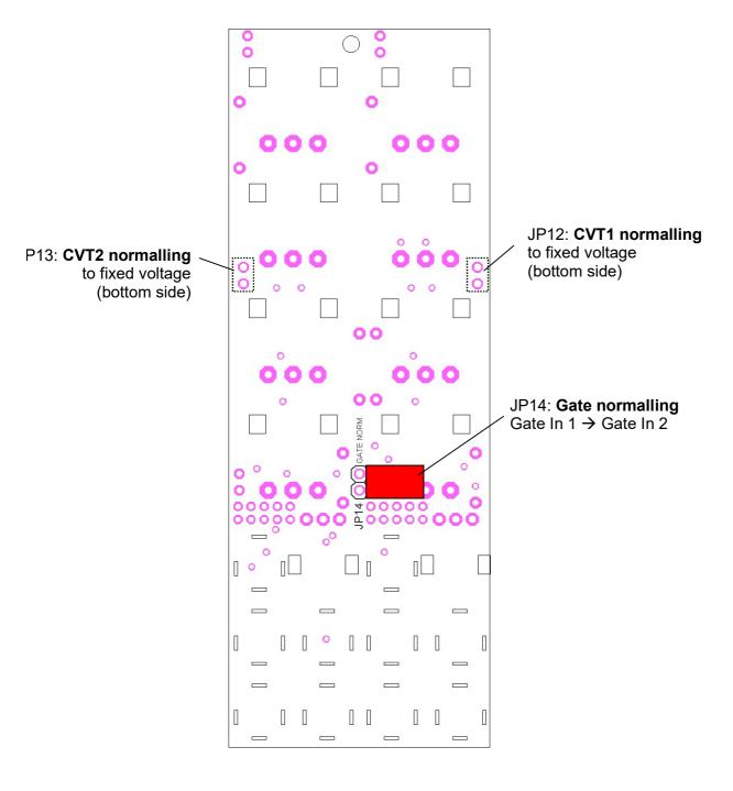
JP14 is an horizontal (lying) jumper and is located on the lower board. To remove or install this jumper a suitable tool has to be used (e.g. a small plier) because it's between the two boards. One may also remove the upper from the lower pc board for easier access. For this the mounting screw at the top of the board has to be removed and the upper board removed from the lower board by pulling out the two 10-pin connectors.
