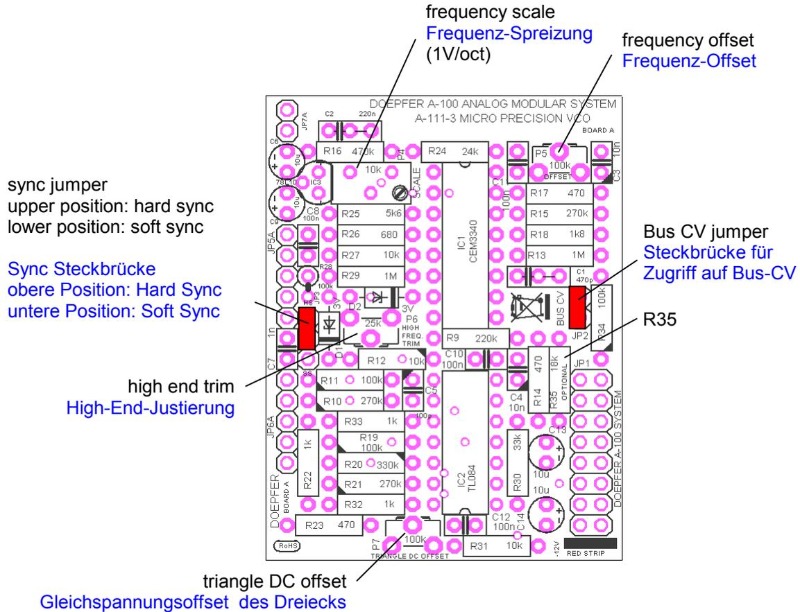
Meaning of resistor R35: R35 defines the DC offset of the sawtooth output. Without R35 the voltage range of the sawtooth output is about 0...+10V, with R35 (18k) the range is about -5V ... +5V.
