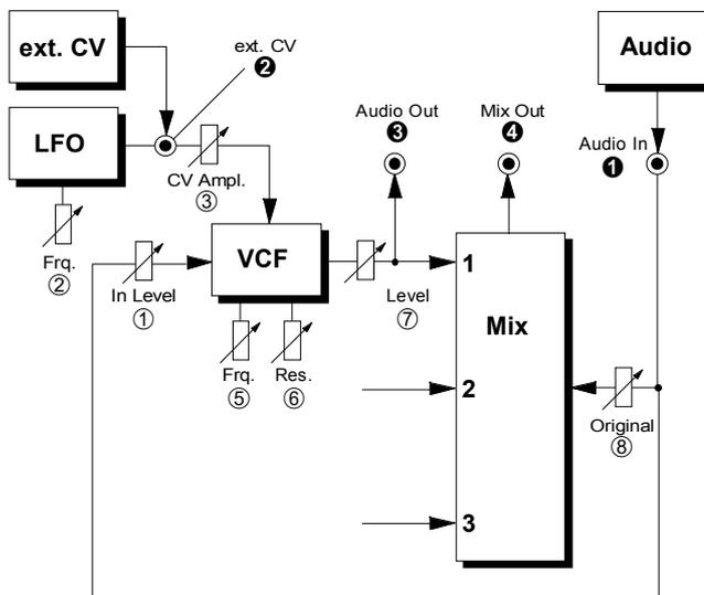
fig. 2: Internal construction of the A-127 (from 1999 output 3 is not affected by the level control 7)
